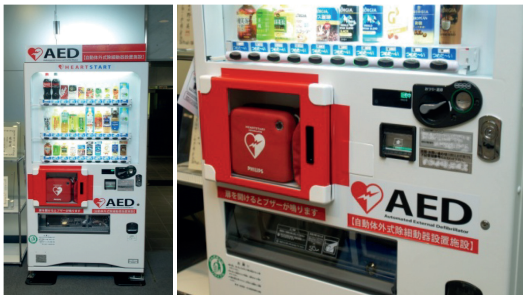
Several million AEDs have been placed as part of AED-Public Access programs. They come most often to use when placed at busy airports and train stations. In Japan AEDs have also been integrated with vending machines.
